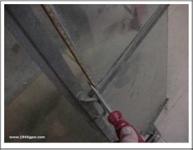
Continue working the glass out...carefully...not wanting to make a big mess with broken glass. I used this screw driver to push the glass out, until it was far enough out I can tap it out with a rubber hammer.
