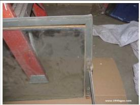
Here, I turned the frame upside down and dropped it carefully on the ground to get the weight of the glass to drop down. My glass is pretty tight so, I wanted to get it started so I can start prying it out.
