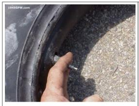
Stuff the flap into the tire around the tube. Pull the stem out, and add a couple of WASHERS around the stem and place the stem cap on the stem so you can pull the stem out. Note: the stem will want to retreat like a turtle pulling his head into his shell.
