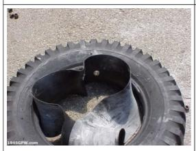
TIP: This part can be a little messy and frustrating. Pre-install the flap on the tube but add baby powder to the flapp so it will slide around. Rubber on rubber does not slide well. Place the stem opening on the tube opening and pull the stem through the flap stem hole.
