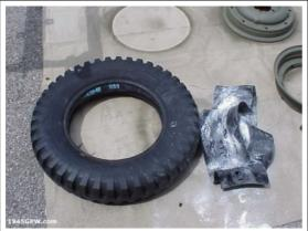
Once the rims have drived completely after a couple days you are ready to install the Flaps, Tubes and Tires. For the first tire install, place the tube in the tire and fill slightly with air. Not much, just enough air to keep the shape up.
