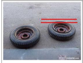
Cleaning up combat rims is a little time consuming. You can do this, while working on another stage of your restore because it is an isolated task. The first thing to do is break the bead on the existing tires. Remove the valve stem to let the air out of tire. Then take another vehicle and run over the tire as shown in read lines.
