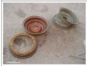
Now the rims are ready for blasting. The rust just peels off with a touch of the hand and should clean up very well.
