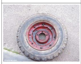
Once the bead is broken on the tire you need to seperate the rims. The nuts are usually rusted on tight. Soak them with penetrating oil. This may take a couple days of soaking each nut on the backside. After each attempt of soaking, you can try and unscrew the nuts.
