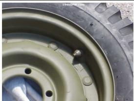
Next, line up the stem with the tube and rim half. Undo the stem cap with washers and pull stem through rim and add screw on the valve stem extender on outside of rim. Then add the other half of rim making sure you don't pinch the flap or tube.
