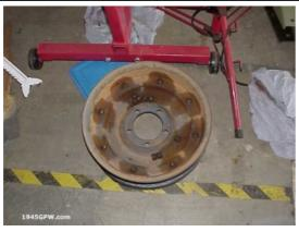
Assuming that you were able to remove the nuts from the back side, you can now take a screw drive and try and seperate the rims. It may need soaking between the rim seam as well. This should come apart fairly easily.
