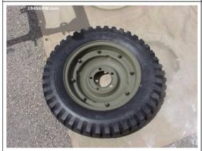
Tighten up the back nuts and fill up with air, and your have completed your first tire install. Repeat the steps for the next 4 rims.
