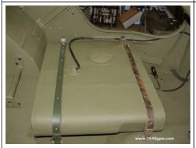
Now install your straps from the channel hooks in the side panel across the tank to the floor hooks. You may need to extend the bolts out as far as they will go in order to line up. Once you have them on, tighten down snug, but not hard as you can dent the thin wall tank.
