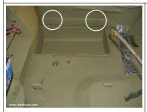
Installing the fuel tank is pretty easy, but the fuel tank straps can be difficult to find. Here we show you the empty tank well prior to the installing of the tank. Circled are the channel hooks that the straps will connect to.
