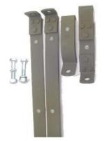
There should be four tank straps an a pair of nut and bolts for the strapping in of the tank. Original straps can still be found at swap meets or ebay, and there are repo sets available as well. The straps have a padding under them so they don't damage the tank.
