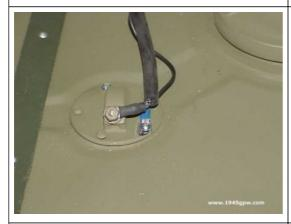
Before installing the straps, you can install the sending unit into the tank. Just drop the sending unit into the small hole on top of the tank and screw into the tank.
