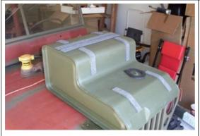
Before installing the fuel tank, flip the tank over and install some padding. There are different ways to do this. G503.com sells thin anti-squeek strips, here you see that a thin strip of Felt will protect the metal on metal rubbing that can occur. This was the example shown by Randy K. on the G.
