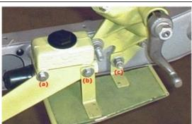
This picture with permission from Ed Campion shows in detail where each of the the bolts will be connected and the master cylinder positioned. From the top view there will be 3 bolts that are appart of this installation. 5/16x18 NC 3" Hex Head 5/16x24 NF 3" Hex Head 5/16 x 18 NC 3/4" Hex Head this one will be connecting to steering housing.
