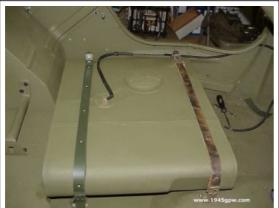
Install the fuel tank into the tub and run the fuel tank lines to the appropriate locations.
