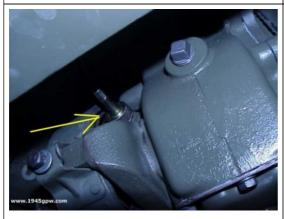
Install the speedometer cable to the transfercase and follow it up through the firewall to speedometer.
