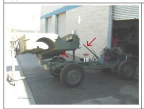
With your tub reading to be mounted, lift the tub up over the steering column (if present) through the floor plate. As you are moving the tub down slowly, follow the steering column forward until the tub is resting on the frame.
