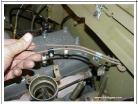
Install the choke and throttle cable on the carburetor. Push the cables through the dash, then firewall and out to the carbureator.
