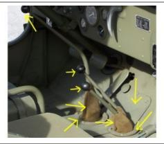
Install the gear knobs and plates onto the floor of the tub. Note: be sure you have the rubber seals for the floor plates
