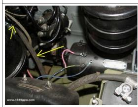
Install the foot starter cable to starter. It is now difficult to get to because tub is on, but you can reach it.
