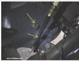
Install the oil line back into the engine block, and connect to the back of the oil gauge in the dash
