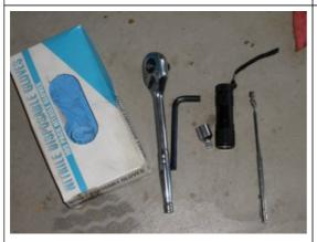
The second set of tools to have ready is the rubber gloves (it will be a little messy), a socket wrench for draining transmission gear fluid, a 3/8" allen wrench for transmission fill plug, and I always keep a magnetic pen ready, so when I drop my plug on the skid plate I can grab it quick.
