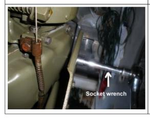
Here I am going to remove the fluid from my transfer case. The plug underneath has a square fitting which a 1/4in socket fits great. Loosen this up and let the fluid out (if you are changing the fluid for example)
