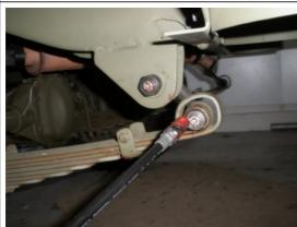
Now back to greasing fittings. On the driver side back spring shackle bolts get zapped both top and bottom.
