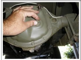
Almost done, now you can put the grease gun down, and check the front axle 90w gear oil. Like the rear axle, remove the plug and stick your pinky finger into the hole and check level add if necessary.
