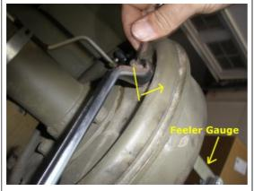
With each wheel, your going to adjust the eccentric adjustments to .008 shoe off the drum. Here you see the feeler guage in the slit of the drum, if you turn the eccentric toward the rim all the way until it is tight, then back it off a bit where you can turn the rim without any rubbing from the shoe, then tighten the eccentric down.
