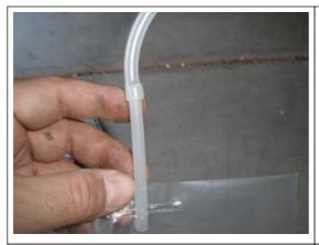
Connect the tube to the retainer bag. Now you are ready to start removing the old bleeders and replacing with the new speedbleeders.
