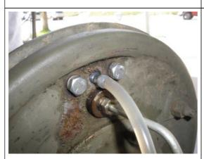
With a closer examination, you can see that the air in the fluid has already been pushed out. Now, tighten the bleeder (clockwise) and pinch the tube off at the bleeder and the fluid will flow down into the retainer bag.
