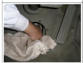
Tip: Clean around the master cylinder and the bleeder, clear area from dirt. You do not want dirt getting into the brake system.
