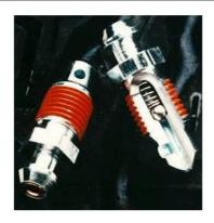
In this article we are introducing SpeedBleeders. No vacuum pump, very simple, one person method using by using www.speedbleeder.com Speed Bleeders. If you look at the picture, you see how speed bleeders work. With the bleeder open a 1/4 turn, and tube connected to the bleeder, a hobbyist can push slowly on the brakes, pushing fluid out, but when your pedal comes up, a check valve will stop air from entering the system.
