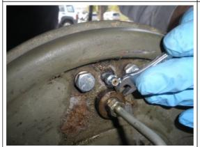
Now, with the old bleeder out, screw in the new bleeder. As you screw in the speedbleeder you might feel a little resistance as you get closer to the end, this is normal as the threads on the speedbleeder have sealer on them.
