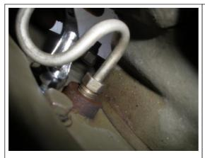
Repeat this process for the other Rear wheel bleeder on the driverside. You will note that the fluid has no more pressure, so the leakage should be minimal.
