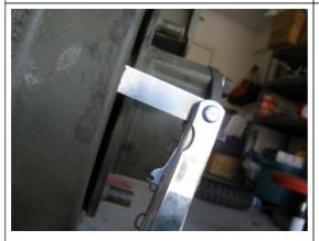
Note on the feeler gauge. The feeler gauge at .008 is very thin. That puts the shoe very close to the drum. You might want to keep the feeler gauge in the slit while testing back and forth. Your margin of error may be greater than .008 so you have to do the best you can between the shoe and the drum rubbing.
