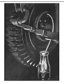
Bleeding brakes can sometimes be very frustrating. With hydraulic brakes you do not want any air in your lines. In most cases, it takes a two people to bleed brakes. One to open the bleeder screw, and the other to pump the brakes.
