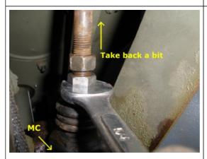
After installation of the speedbleeders you might find that your brake pedal goes to the floor. If so, you need to adjust your brakes now that all the air is out of the lines.
