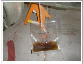
I moved to, and finished the passenger side front wheel and I was looking at the amount of fluid I now had in the retainer bag. At this point you want to check your master cylinder fluid level. I added more fluid to the master cylinder because you don't want the cylinder to go dry and get air back in your lines.
