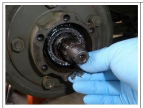
Next, find the notch on the bearing lock washer and align it on the axle shaft and push all the way back so it sits next to the cone bearings.
