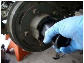
Then tighten the bearing nut with your wrench so it is nice and snug. Use a screw driver in the wrench notches to tighten this nut on securely.
