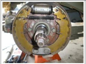
Assuming that you have removed your Front Brake Drum already, we now want to replace it. Before you begin, it is recommended to Pack your Bearings. You should be ready with to install your drum over the brake pads
