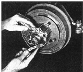
Measure for SHIMS! As you see in this picture from the TM, put your flange back on and screw on the axle shaft washer and nut. Continue to screw on the castle nut by hand until you see the proper placement for the cotter pin through the castle nut hole.
