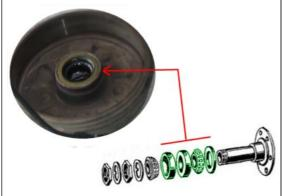
If you are re-installing the front brake drum, the back side of your drum should have some components already installed as shown here, if not consult the TM-1513 and install them. It is a good idea, to remove these items and re-pack your bearings while your drum is off.
