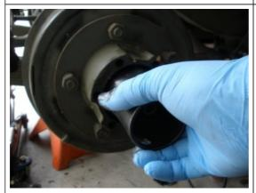
With your wheel bearing wrench, hand tighten the nut on the wheel. TM-1513 recommends to tighten the nut until you start to feel drag when you spin the wheel. In many cases, you may not feel any drag. If you have it on tight or if you feel a little drag, the TM recommends that you bring it back 1/4 turn. The drum should NOT have any play in it when moving back and forth.
