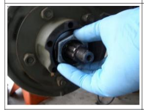
Next, install the last bearing nut with your fingers all the way back against the lock washer. If you try to wiggle your brake drum it should have no play in it.
