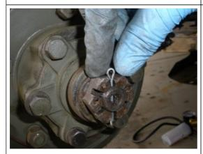
Then install the axle shaft/flange castle nut. The castle nut should tighten down past the hole for the cotter pin, to to far.
