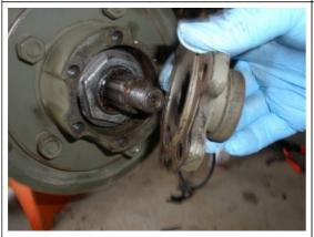
Now align the shims on the flange and install on the axle shaft.
