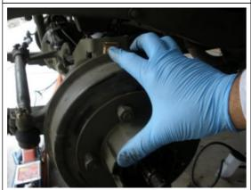
Spin the drum again and try and wiggle it, should be secure with no play.
