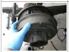
Assuming your are ready to re-install, push your Front drum carefully over the axle shaft and over the brake pads. You should feel the drum move all the way back on the axle over the brake shoes.
