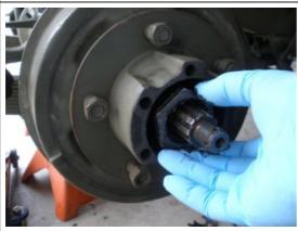
Apply the wheel bearing nut with your hand screwing it on as far as you can with your fingers. Your drum should still be all the way back on the axle
