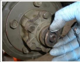
Next install the axle shaft/flange washer
