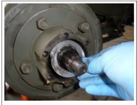
Install the 2nd lock washer on the axle shaft, with the notch lined up on the shaft as you did the previous one. Push all the way back against the nut.
