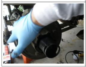
Once you think the nut is on correctly, spin your drum (should be out of gear of course), and you see and hear the drum move freely.
