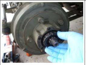
Next, install your cone bearings with the pointy end first (see diagram above). Push them all the way back into the drum.
