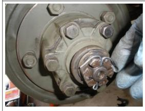
Bend the cotter pin around the axle shaft nut as shown.
