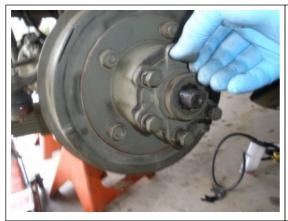
Press the flange all the way back and install the flange bolts.
