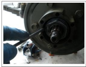
With a screw driver, bend the lock washer out so it has a little lip on it to keep the outside bearing nut from revolving.
