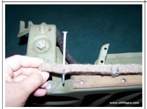
You can use an Ice pick or a long nail to poke holes into the felt. I didn't have an ice pick, so I used a large nail and pushed the nail through. Lay the felt up on the grill and see where it should align with the markings and place your nail on that spot and push through. Make sure you have it lined up straight across the grill shroud. The felt is really think so this takes some doing.
