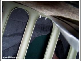
I pushed the staples through the holes of the felt. The felt is thick, so you have to push it as far as you can, otherwise you won't find it on the other side. Use your needle nose pliers to line up the ends of the staples to the holes and push through.
