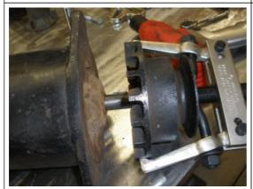
Use a puller to pull off the front pulley as shown.
