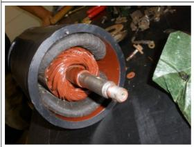
To test that we have the field coils on tight enough, we insert the commutator into the field coils. The first time we did this it was too tight. Then we cranked down the field coils screws some more, then it would turn freely. With the new taping, we expect it to be very tight.
