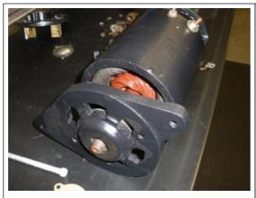
After the Commutator is in the housing, Place the Drive End plate over the Commutator shaft. It will be snug, apply some assembly lube if needed to slide it on. Line up the holes in plate with the shafts sticking out of the housing and tap on tight.
