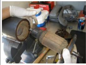
With the front and back covers off the housing, the commutator should pull right out.
