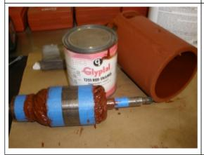
Next, we primered the generator casing, and now we are going to insulate the commutator wiring and the inside of the generator casing wall. We use the popular, but hard to get in California "Glyptal" insulating red enamel. This insulator is to help water proof your generator wiring.
