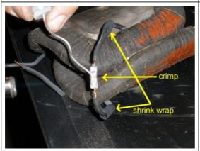
Here we repaired the broken wire between the field coils. We used a crimp first, then soldered it together. NOTE: we prepared the shrink wrap before we crimped the wire and soldered. Also, let the solder cool down before trying to apply shrink wrap
