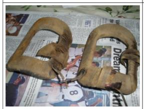
Placed on newspaper because it will be a little messy, seperate the field coils carefully. Want to be careful to keep not tear up the fragile wires.
