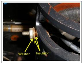
After inserting the field terminal through housing, install the cylinder insulator and circular insulator around the bolt, then washer and nut as shown. Tighten down, BUT NOT too tight! just enough to hold firmly against housing.
