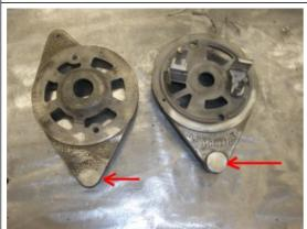
In our 220 welder we have a good hard steel, so it looks like the welds will stick. We filled both the holes via welder and grinding them down. We will center the position and drill a new 5/16in hole.
