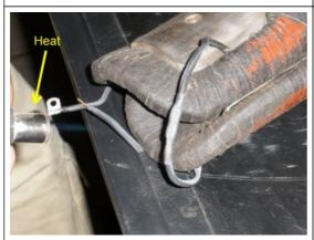
Here we show the 2nd shrink wrap over the crimp and we applied heat with a micro torch. The field coils are now connected back together and insulated.
