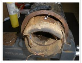
With the field coils two screws removed from the housing, gentley remove the field coils by pulling them out. Note: they are connected together. Be careful not to break the connection when pulling the field coils out.
