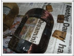
Tear a piece of electrical tape, enough to wrap it twice around the coils. Carefully, wrap tightly around the coils. Note the position of the connecting wires as you want them to be in the same exact place as they were before.
