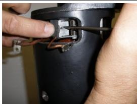
With the spring pulled back with the hook pick, slide the brush into position. The brushes can only go in one way correctly, and with the wire in the down position it should slide in very easily. When you let the spring back, it will snap into place.
