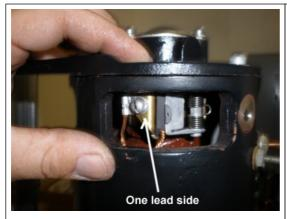
Now attach the brush leads to the spring assemblies. Starting with the side that only has one wire from the brush, attach it to the spring assembly as shown. These screws are included in the NOS kits.
