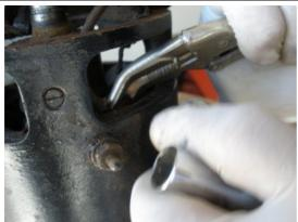
Disconnect the terminals from the casing. There are three connections that you will need to disconnect, so take your time and carefully disconnect each of them as the wires are brittle.
