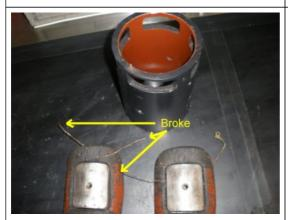
At this point we need to prepare the field coil wires to be re-installed. In this case, the wire insulation has crumbled and the the wire between the field coils has broke. So we need to fix these items.
