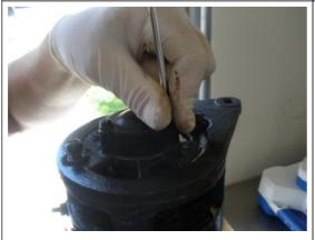
Remove the commutator cover plate screws from the back cover plate of the generator.
