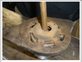
Remove Bearings: Now we move back over to the housing covers which hold the bearings. Start with the pulley side cover plate. Here we place the cove over an over sided cylinder. Take a tap, and tap the bearing out of the center of the cover plate.
