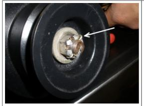
Install the cotter pin around the castle nut. NOW, you can spin your generator CLOCKWISE to verify it is spinning freely. DO NOT spin counter clockwise. You should feel a little resistance, but nothing rubbing. This one feel very good.
