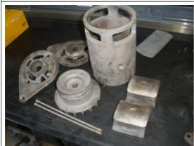
All parts that can be sandblasted are completed. Next we are going to fix some of the areas that need restoring.
