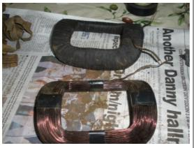
Now repeat the same steps on the other coil. Start with unwrapping, and replacing the four point paper wrap with electrical tape.
