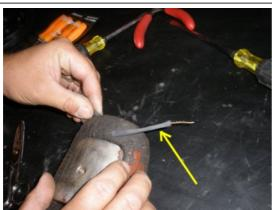
The first thing we want to do is to insulate the wiring again. Here we are preparing some Heat Shrink wraps around the wire. We measured the wrap and cut it slightly shorter than the end of the wires.
