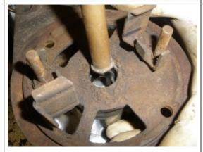
With all the wires disconnected from the rear plate, we can pop the bearings out of the center of the plate as we did with the front cover, that is, with a punch and tap it out.
