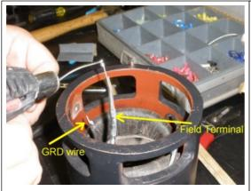
Here you see we dropped the field coils into the housing to see how much wire we had to work with on the Field Terminal. The Ground wire did not need repair so we are ok, but the field terminal needs to be reconnected. Here we prep the wire with some solder.
