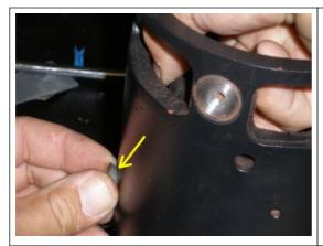
Here you see Harley applying new NOS screws to the outside of the generator housing. We had to drill these out earlier. You must really crank these down in order for your armature to be able to turn.
