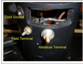
Tighten the armature washer and nut down firmly to the housing. Again, be careful not to tighten down too tight.
