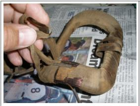
Unravel the tape carefully. The coils are held in place by four strands of a paper tape that will most likely come apart as you are unraveling. You don't want the coils to fall apart, so have your electrical tape ready to replace.
