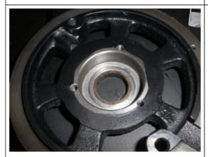
Lets start with the Drive End Plate, Place the felt washer in first around the center hole, and tap your retainer ring into position, when the retainer ring is secure, you should see the felt washer through the center of the plate as shown.
