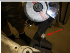
Here you see the head is filled with a weld and grounded to its original shape, and we prepare to create a new slot with and angle grinder.
