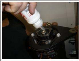
Now prepare the Commutator shaft with a little assembly lube so the bearings will slide on easily.
