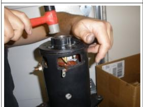
Now, install the Commutator End Head plate on to the housing. Like the other plate, this should line up with the studs out of the housing and will most likely be a little snug. Tap on if needed for a tight fit.
