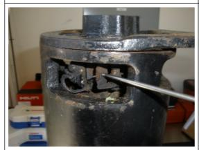
Next, we want to disconnect the brushes. Find a hook type device that will allow you to pull back the brush springs as shown here.
