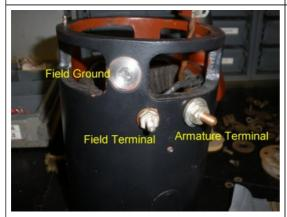
From the outside of the housing, your see Armature and Field terminals and field ground
